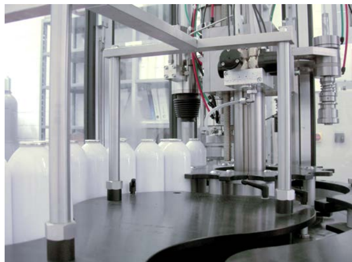
Fully automatic filling of pressure cans
